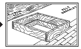
**STEP 2:** Fit sheet metal flashing to the curb surfaces with a 3" flange around the base and a 6" flange on the uphill side. Corners should be overlapped and edges joined with tabs. Seal the top and under sides of metal flanges with roofing mastic.
