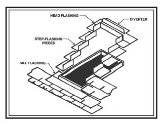
**STEP 3:** Continue to install shingles. Apply a bead of caulking on top of curb around the perimeter. Set the skylight down, fasten with No. 14 cadmium-plated wood screws.
