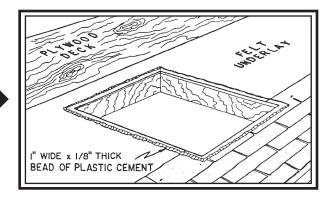
**STEP 2:** Center the skylight over the hole and nail it to the roof with roofer's nails. Nail in the hole provided in the flange. Place another bead of plastic cement on top of the skylight flange at the sides and the top as indicated in the drawing.
